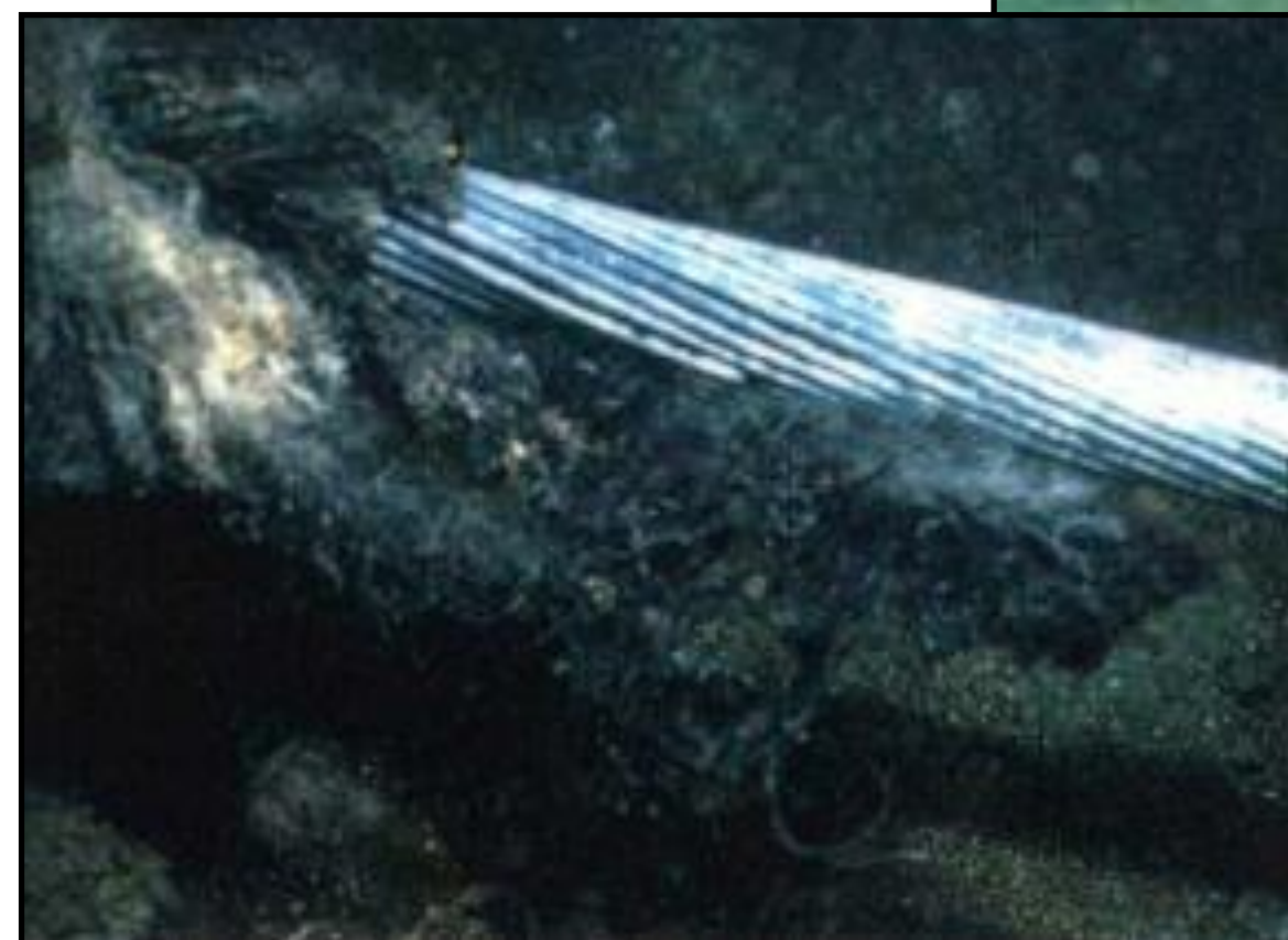
Cable damaged by trawl gear
