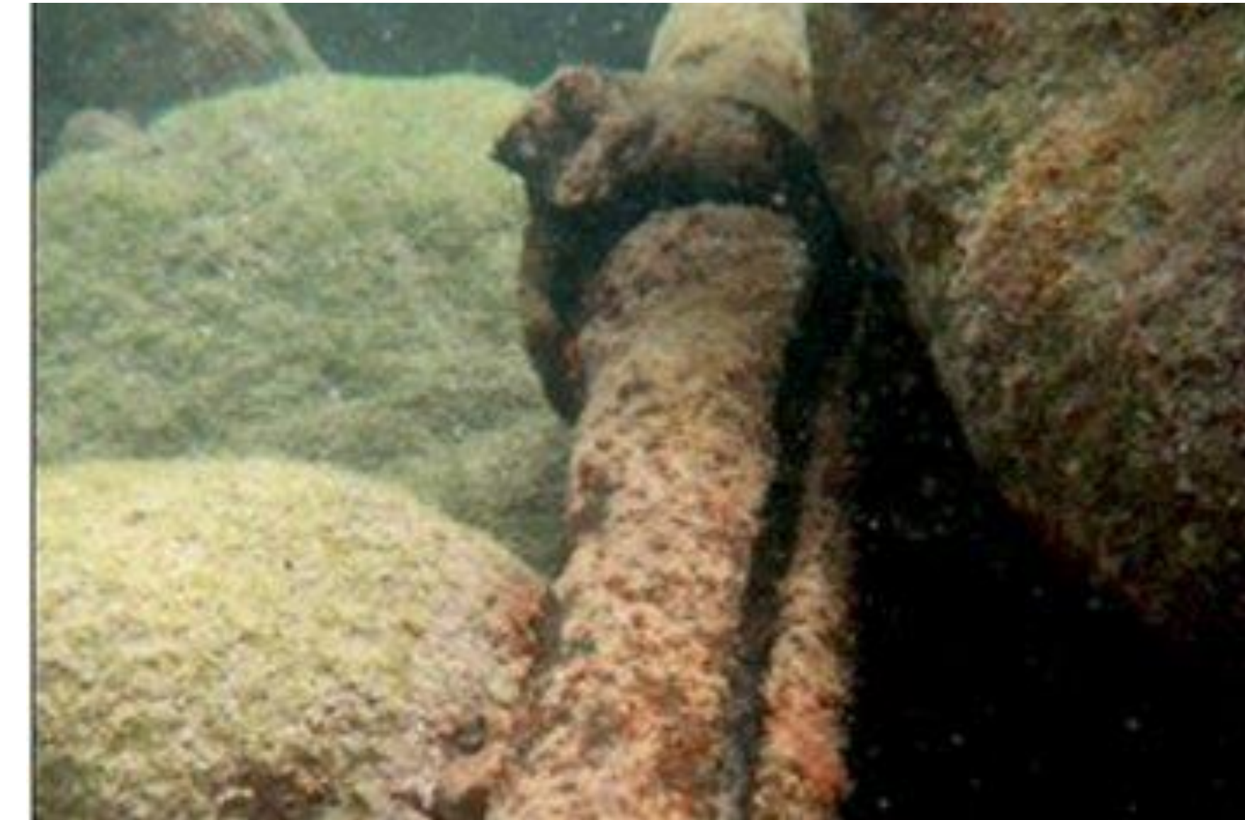
Subsea cable damage caused by shifting sea bed conditions
