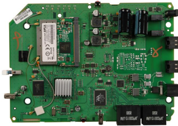
Livebox V2: Wi-Fi functionality on daughter board, connected with Mini-PCI
