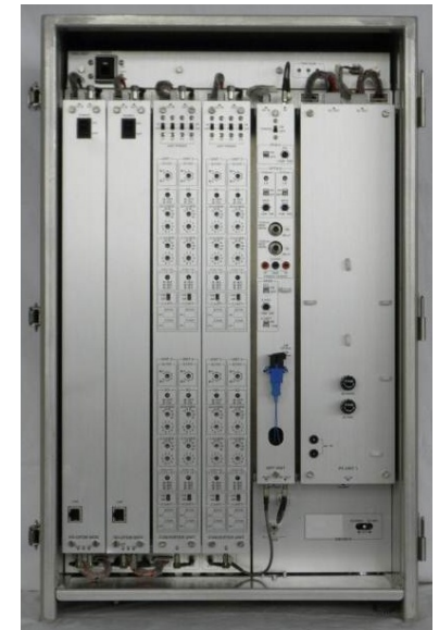
Developed portable provisional headend equipment
