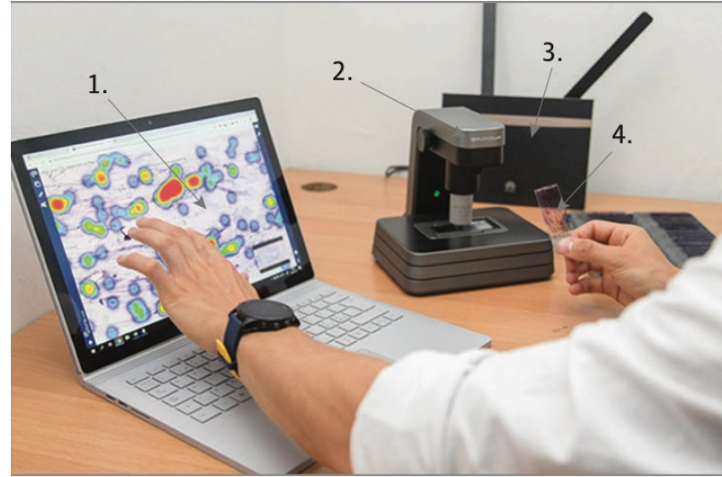
Slide digitization equipment, including (1) laptop computer with access to the slide- management platform, (2) slide scanner, (3) mobile-network router, and (4) Papanicolaou test microscopy slide
