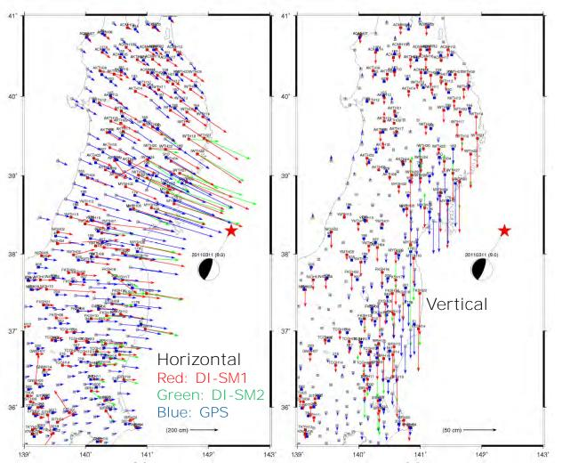
Obtain static displacement through double integration of accelerometer records (after correcting for accelerometer drift)
