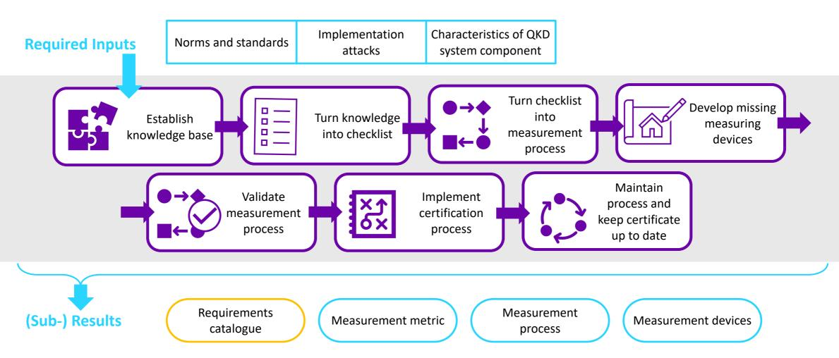
Based on research results, an evaluation process for certification of QKD system security can be created.
