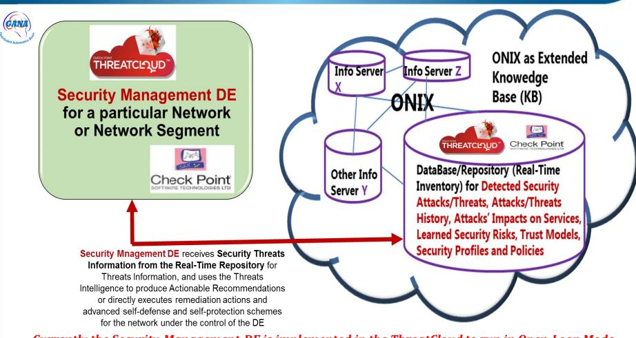
*Currently the Security-Management-DE is implemented in the ThreatCloud to run in Open-Loop Mode but can be made to run in Closed-Loop Mode.*
