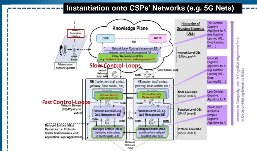
GANA is a Model for Multi-Layer Autonomics & Multi-Layer AI Models & Algorithms Some MEs of an NE, such as Protocols of the Stack, may have own intelligence for security enforcement or may intrinsically embed security features. However, the MEs communications with the outside world may need to be constrained or policied (policy-controlled) by the global security enforcement policies of the NE's Security Management-DE
