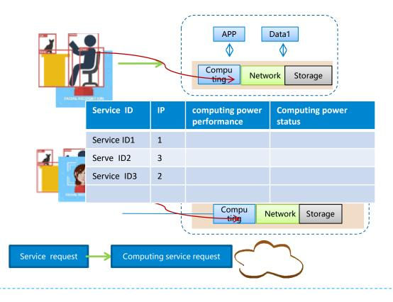
**Computing and network collaborative scheduling**: according to service requests, dynamic task dispatch is performed in combination with network status and computing resource status.
