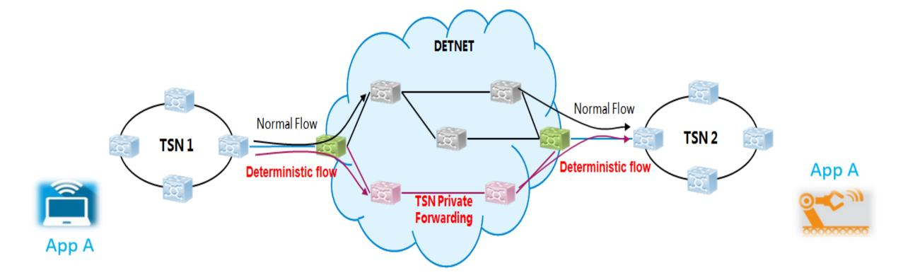
Scalability of DetNet in large-scale networks including stateless of traffic forwarding, no need for precise time synchronization between devices is beneficial for DetNet applied in the industry.
