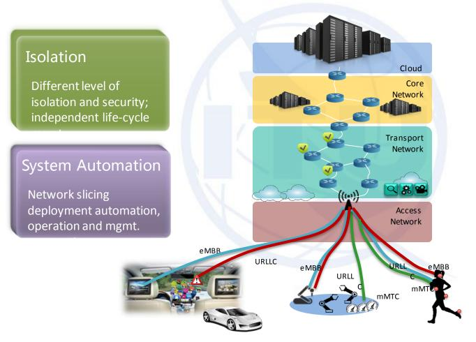
Network Slicing is E2E It includes Terminal, AN, TN, CN and Cloud.
