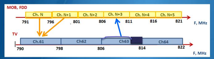
Multiple interference from several station into one receiver -> aggregation of interference (power sum, Monte-Carlo, etc.)
