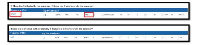
"What if" study, showing incompatibilities simulating the assignment of a frequency to the wanted station, scanning through the whole FM band in steps of 100 kHz. Below the analysis of FLEX against FLEX requirements, the tool presents, for each frequency in steps of 100 kHz, the following information
