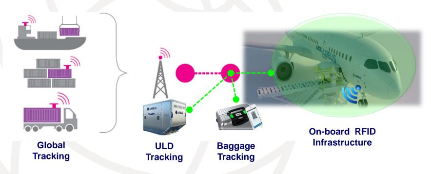
ULD: Unit Load Device, RFID: Radio Frequency Identification, WLAN: Wireless Local Area Network
