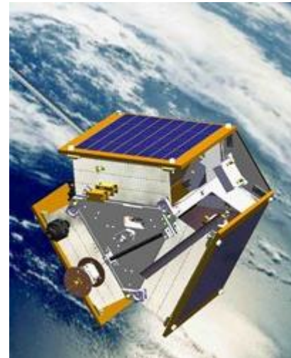
SNAP-1, 6.3 kg, butane propulsion system
