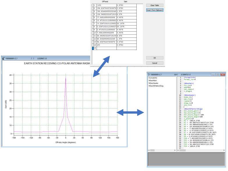
Enter points using the digitiser or by typing on the keyboard
