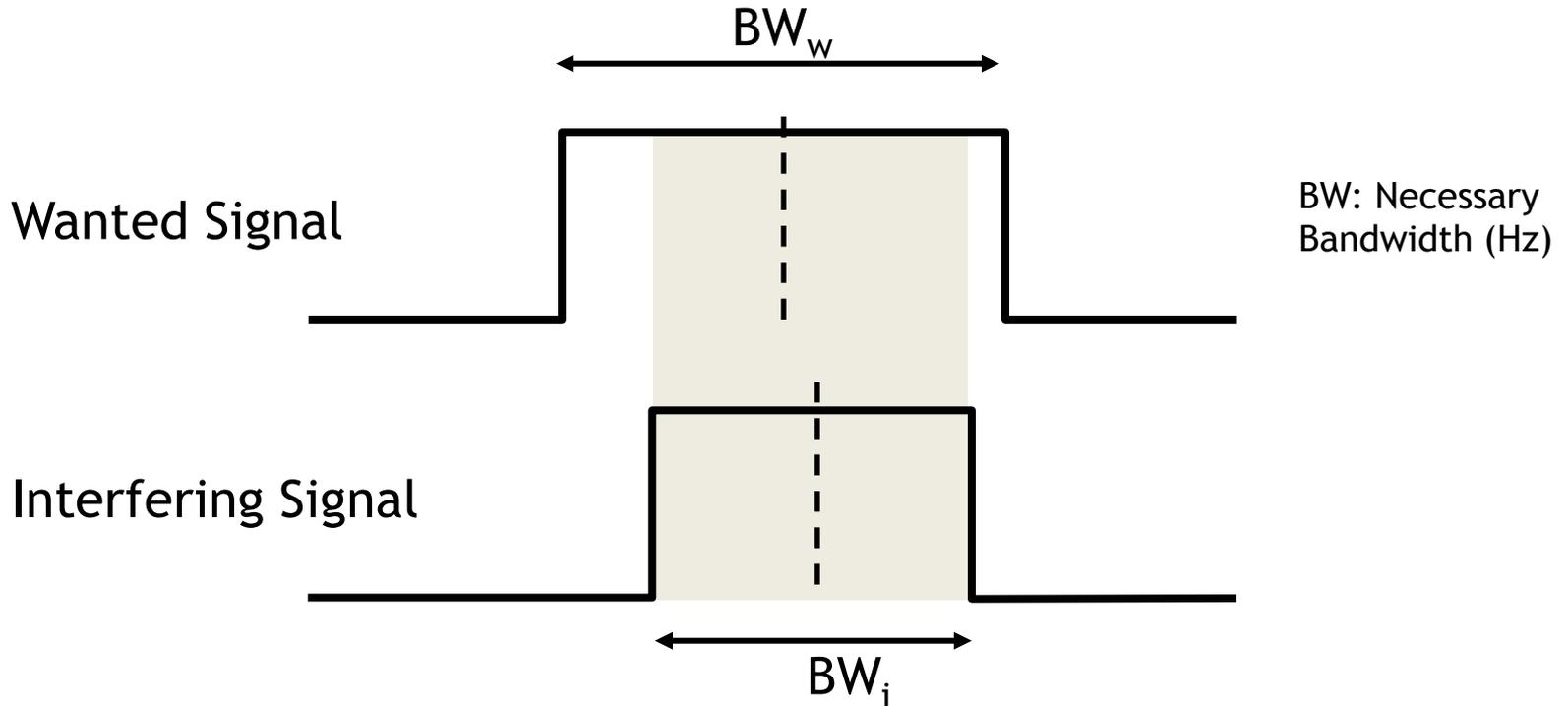
$$\begin{aligned} I_a &= 10\log_{10} (BW_{\text{overlap}} / BW_i) \\ &= 10\log_{10} (BW_i / BW_i) \\ &= 0 = \text{No Improvement!} \end{aligned}$$
