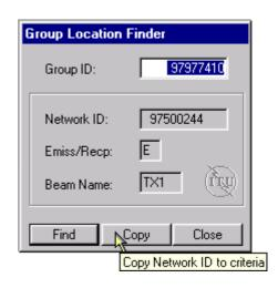
At this point the utility locates the corresponding network information and displays the Network ID, Emission / Reception flag and the Beam Name as shown above on the right. To insert the Network ID value into the *BR Network ID* criterion field on the *General Criteria* tab, click on the Lopy button.
