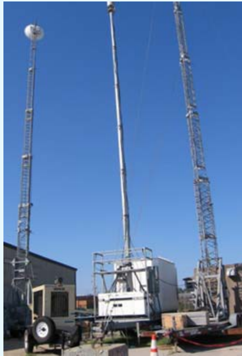
Figure 3-18: Sprint-Nextel's COW (middle of the image) and portable transmission site
