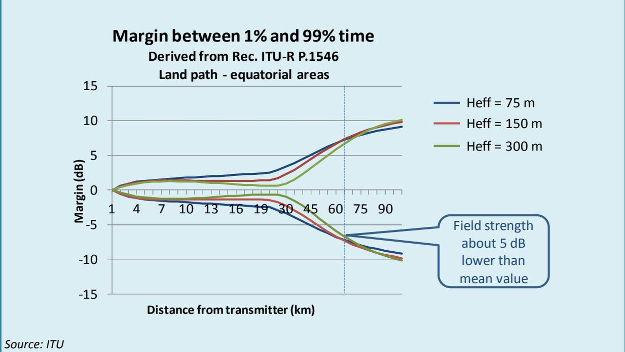
Figure 34 shows that up to about 25 km from the transmitter the time variation is relative small. At larger distances the variation increases and is about 10 dB higher than the mean value for 1 per cent of time and about 10 dB lower for 99 per cent of time<sup>61</sup>. The frequency planner is faced here with the question of what an acceptable variation is.
