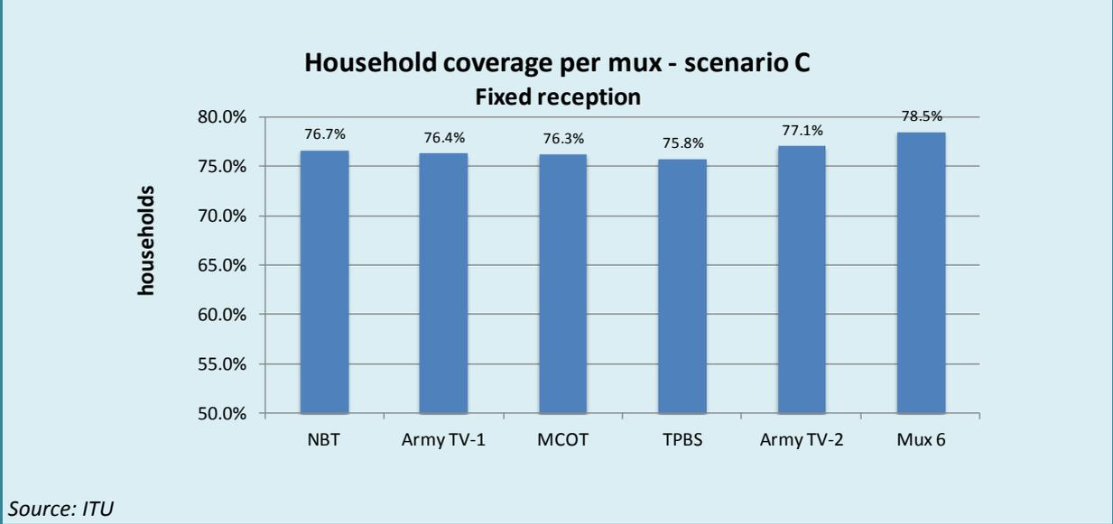
The household coverage ranges from about 76 to 78 per cent. The differences are minimal between the multiplex and are mainly caused by propagation differences between lower and higher channels. In multiplexes 1 to 5 the channels per site were arranged to obtain equal coverage per multiplex. Multiplex 6 contains many channels in the lower part of the band, but was excluded from this arrangement, because most channels in multiplex 6 are in operation by Thai PBS analogue TV (in scenario A and B).
