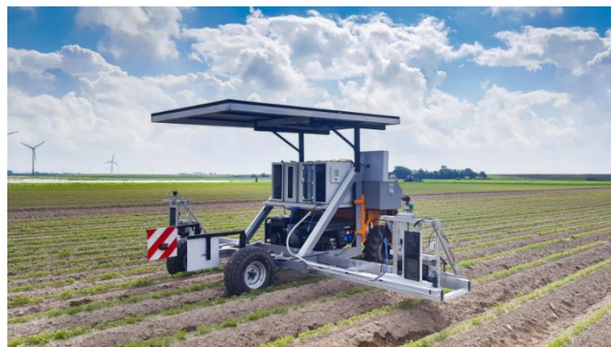
8-Track Weeding Robot during a field test / Credit: Naiture GmbH & Co. KG
