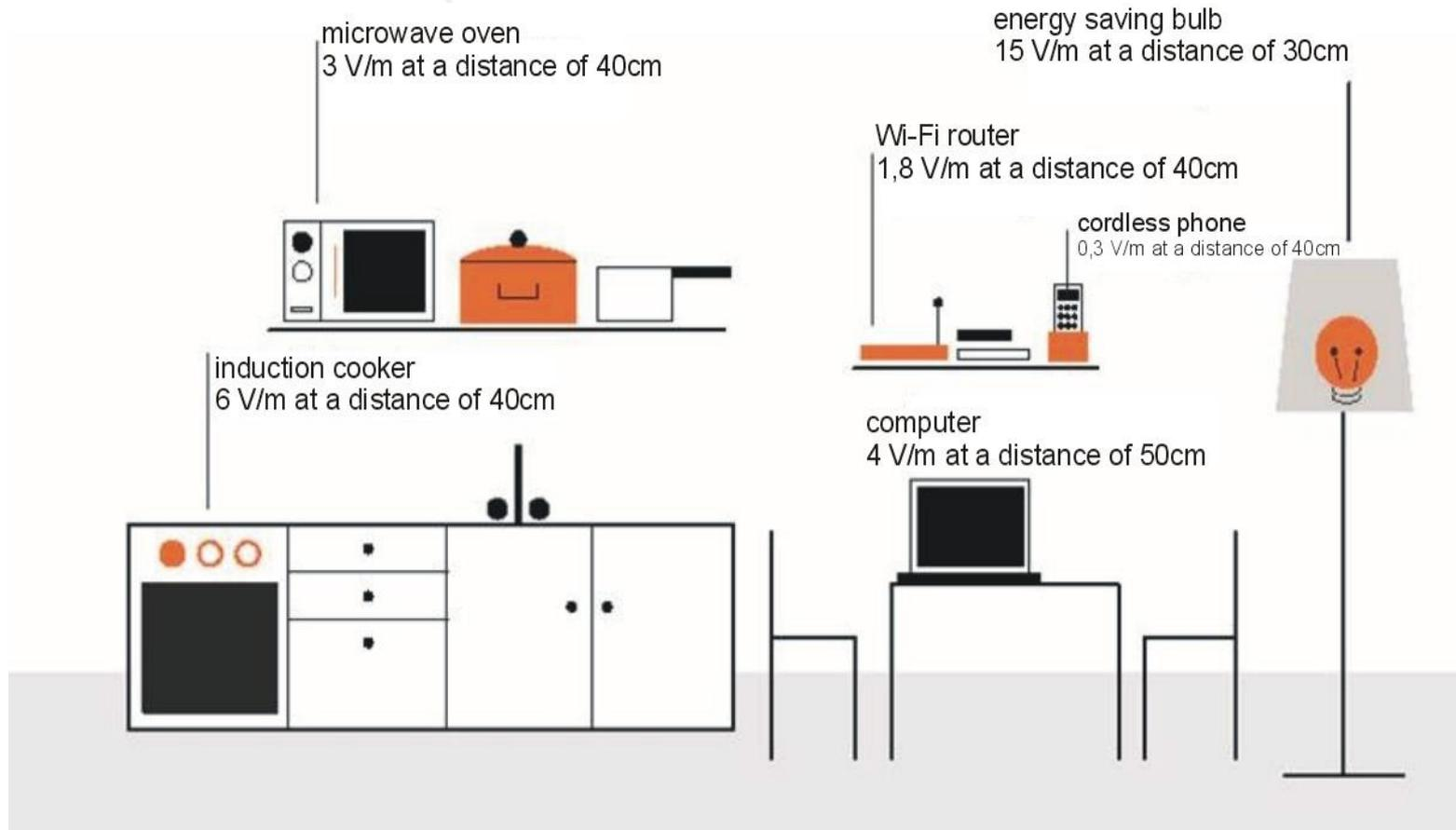
Exposure levels around typical electronic and electric equipment in home environment
