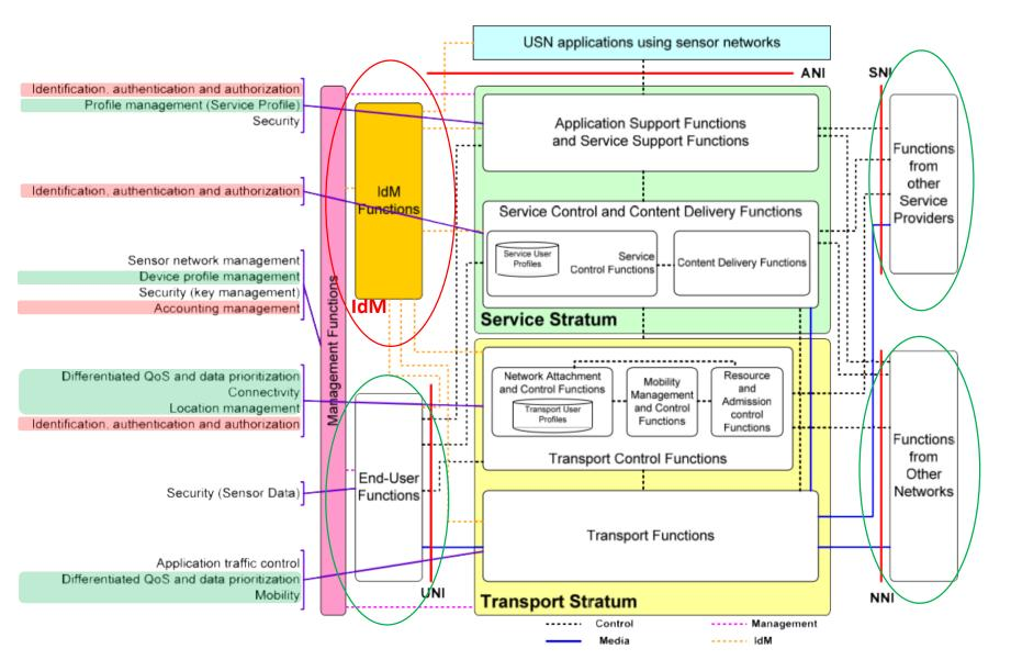
Recommendation Y.2026 (12) Functional requirements and architecture of the next generation network for support of ubiquitous sensor network applications and services
