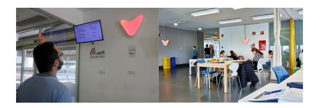
Visualfy Places is an artificial intelligence system that mimics the human sense of hearing, recognizing relevant sounds such as a fire alarm, a doorbell or a baby crying, among others, and translating them into visual and sensory alerts in any chosen connected device, like smart bulbs, a smartphone or smartband, allowing deaf people to react to them, and offering an inclusive user experience in public buildings.
