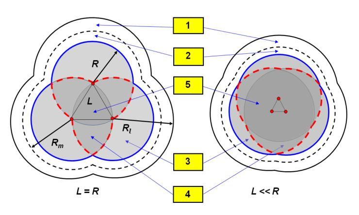
Various monitoring coverage zones under different ratios of distances between stations (L) and DF coverage area radiuses (R):
