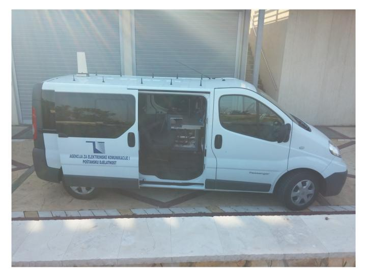
Digital mobile control-measuring station Renault Traffic Passenger (DMCMS)
