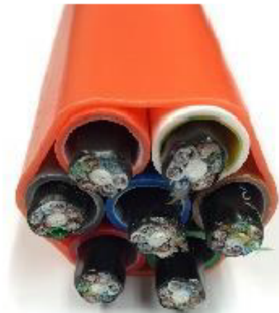
288-F with 200 \mu m SM 8.0mm (O.D.) in 10 mm (I.D.) micro-duct 11
