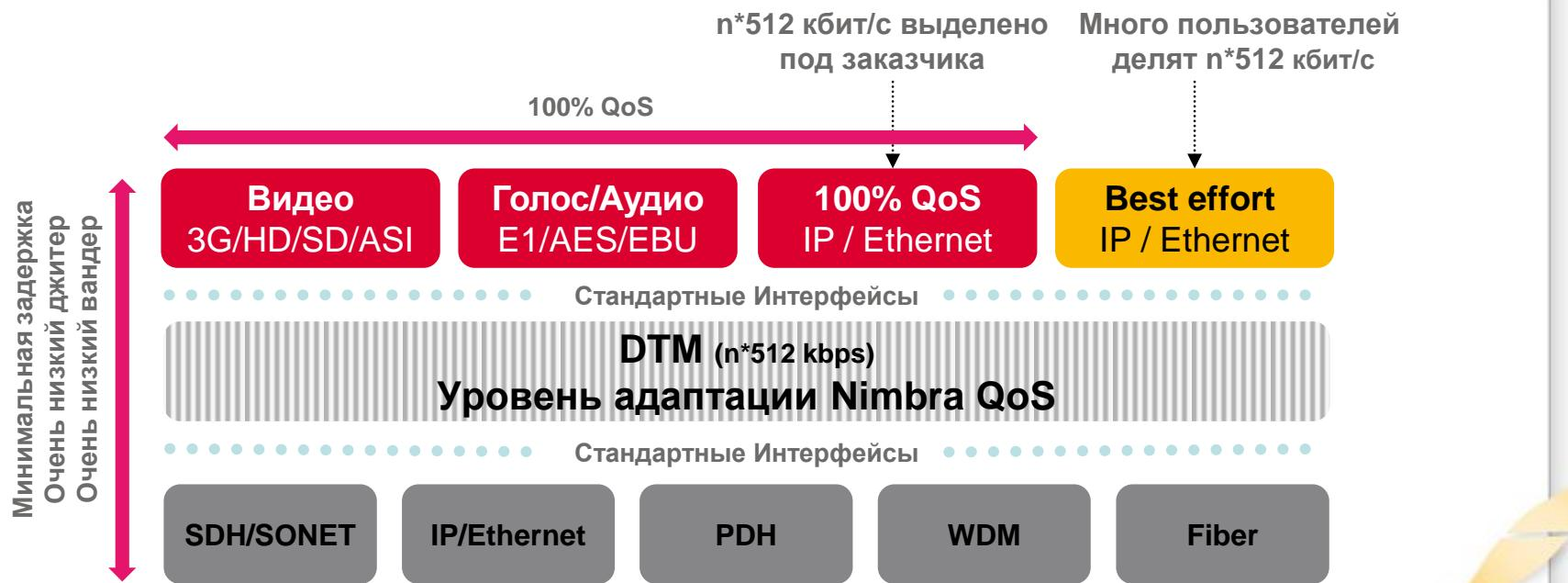
DTM (Dynamic synchronous Transfer Mode) - Стандарт ETSI (ES 201801-1)
