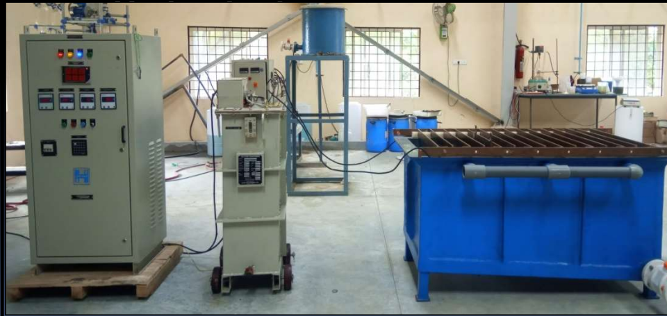
Electro-Refining unit (5kg/day Deposition rate)
