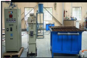
Electro-refining (5kg Cu/day)
