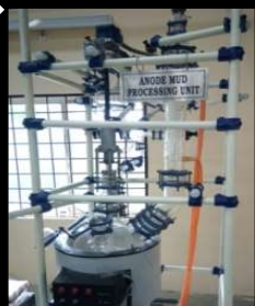
Anode mud processing (5kg/batch)
