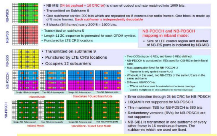
Maximum Transmission Block Size = **680 bits** Inband mode: **100 to 108 symbols** – Standalone/Guard band mode: **152 to 160 symbols**
