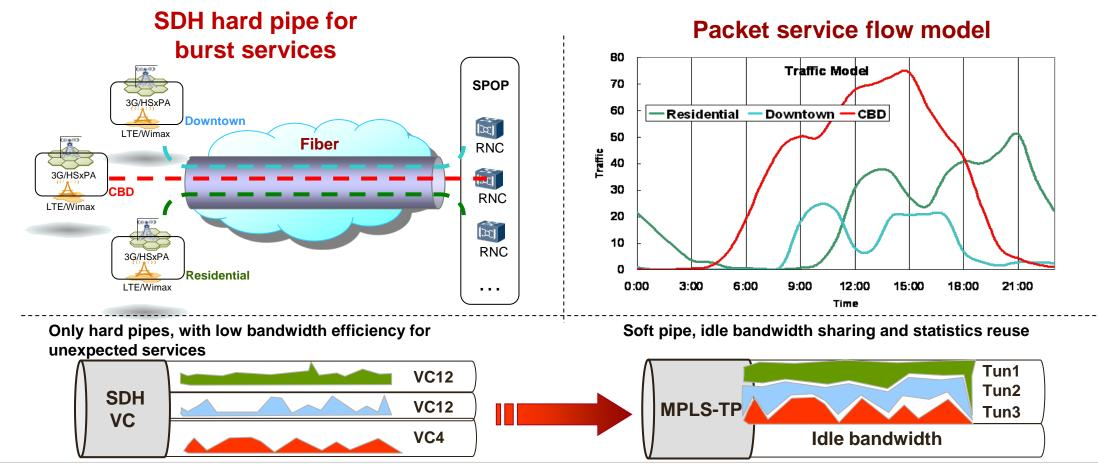
The VC pipes of SDH/MSTP use exclusive bandwidth, and the bandwidth efficiency is low during packet service bearer.
