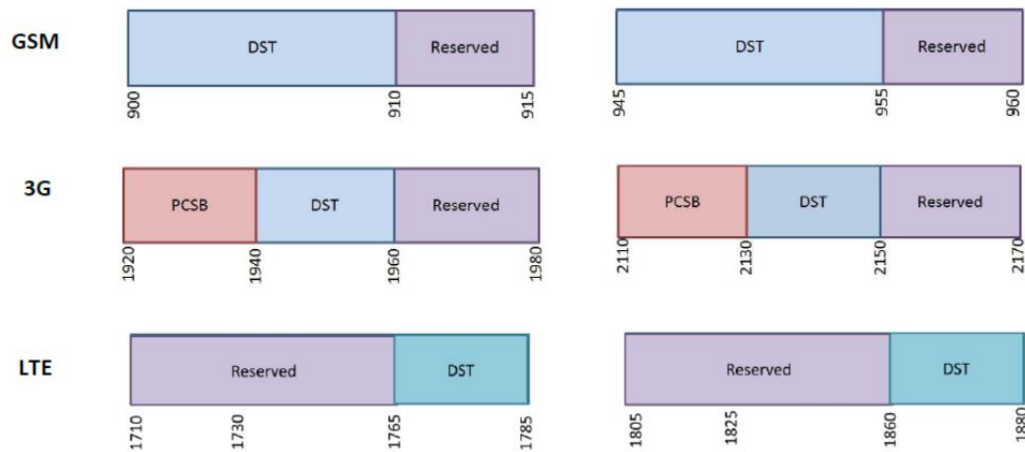
Figure 3.1: The cellular mobile band allocation in Brunei Darussalam
