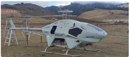
Unmanned helicopter with public/private networks and EO/IR pod
