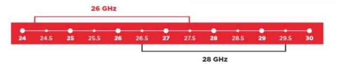
3GPP band n258 refers to the range between 24.25-27.5 GHz and is commonly called 26 GHz. And 3GPP band n257 refers to 26.5-29.5 GHz. It is commonly called 28 GHz.
