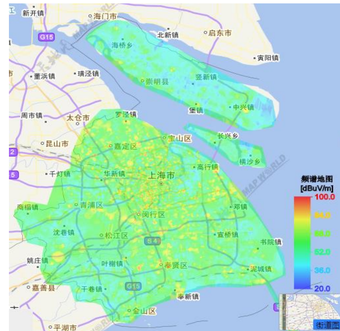
Field Strength of a Frequency Band (934MHz-936MHz)
