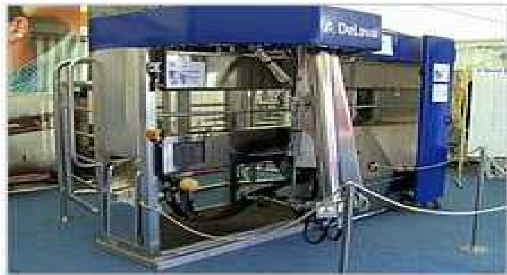
DeLaval milking station
