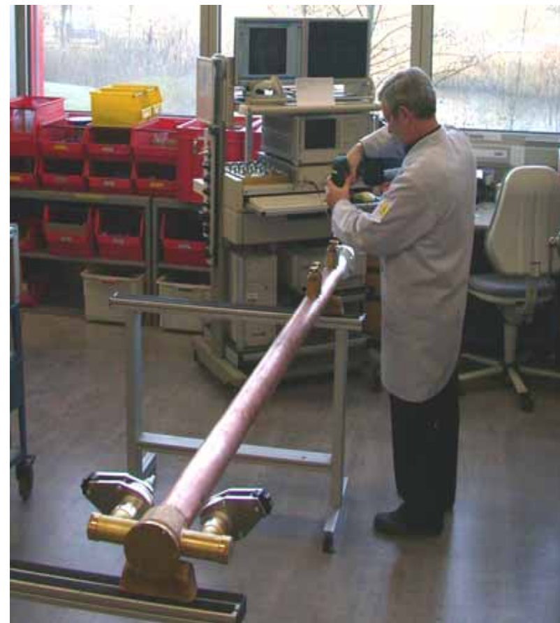
Example: VSWR-Test of Power Splitter
