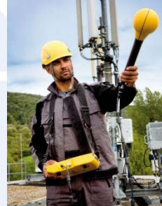
Frequency selective meter dedicated to EMF, with isotropic-antenna
