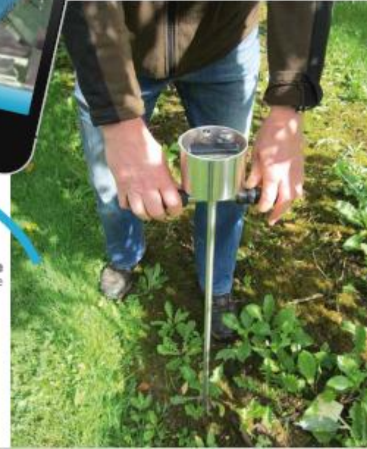
TDR Probe measuring soil moisture
