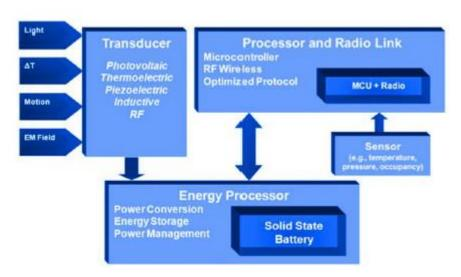
Energy harvesting - components of an autonomous wireless sensor (Source: Cymbet)
