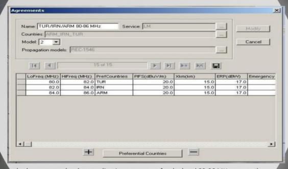
The example shows a cross border coordination agreement for the band 80-86 MHz among three administrations. Three sub-bands are established, one for each country, giving preferential assignment rights. The limits of the preferential rights are 20 dbuV/m measured at 15 km across the border. For coordination of receivers, a reference transmitter with e.r.p. of 17 dBW is used.
