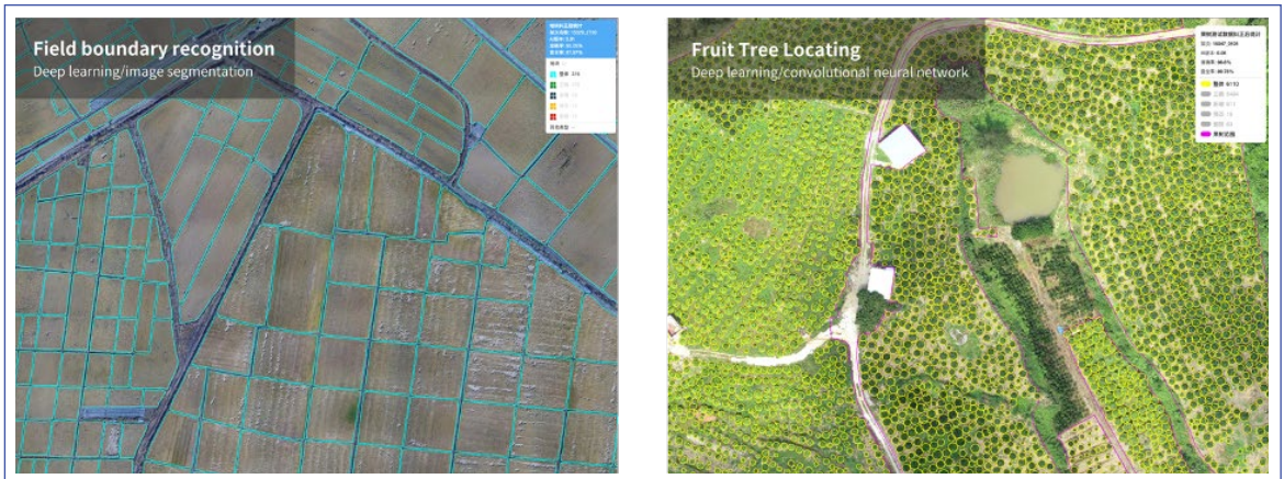
Picture 6. XAG artificial intelligence identifies field boundaries and fruit tree location for field mapping
