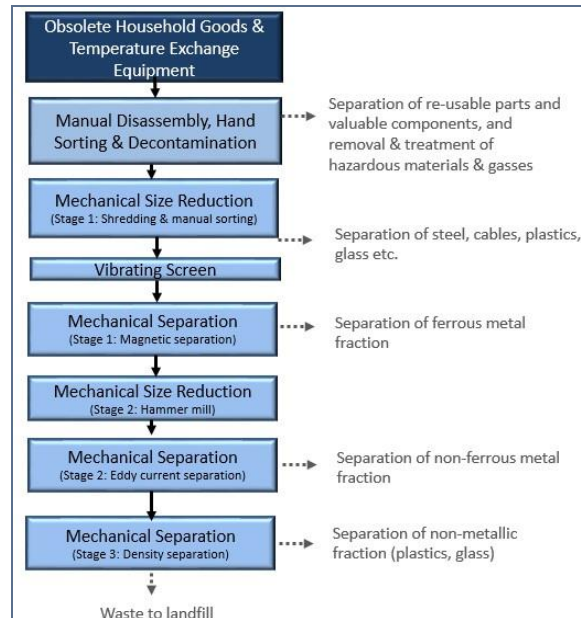
Figure 6: Simplified flowsheet for household and temperature exchange equipment recycling
