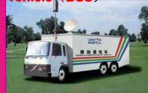
Mobile base station vehicle (BSS)
