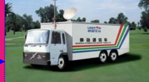
Mobile base station vehicle (BTS)
