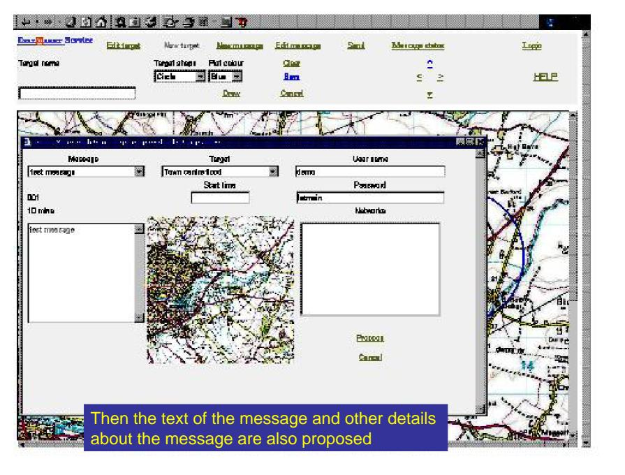
If the Broker sees that all policy has been followed, then it is reformatted and Signaled to each network in turn. It is then broadcast to all mobiles camped On the affected cells, which then alarm and display the message.
