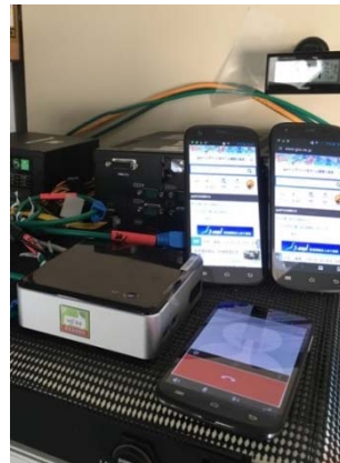
MDRU with NICT's vehicle-mounted satellite base station
