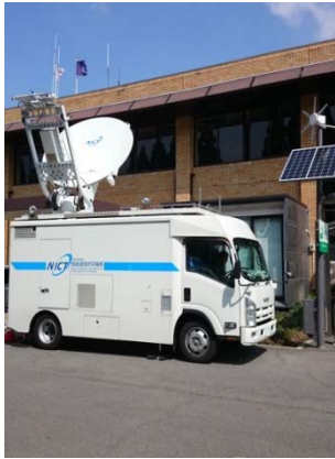
MDRU with NICT's vehicle-mounted satellite base station
