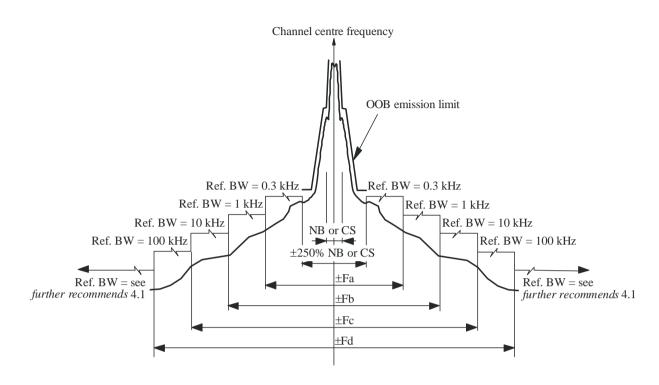
Note 1 – ±Fd frequency steps are not applicable if lower than 1 GHz. ±Fc frequency steps are not applicable if lower than 30 MHz. ±Fb frequency steps are not applicable if lower than 150 kHz.
