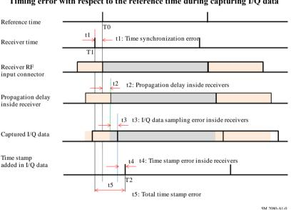
FIGURE A1-1 Timing error with respect to the reference time during capturing I/Q data
