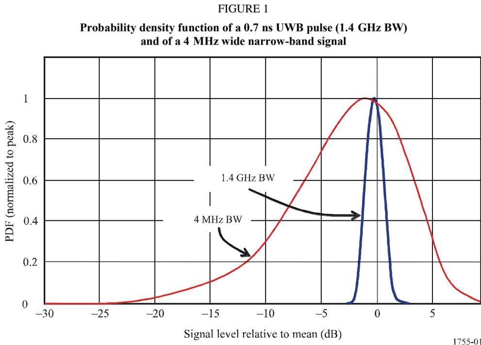
During propagation a sub-nanosecond pulse is dispersed, which may result in Rayleigh fading in the frequency domain. However, each of these reflections is an independent signal so a RAKE receiver can then be used to coherently add the energy in each of the pulses that are received from each of the multipath components to provide a gain over single path reception.
