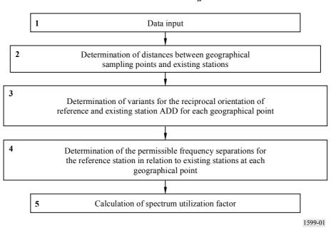
FIGURE 1 Consolidated flow chart for the algorithm method
