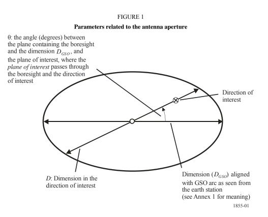
NOTE 1 – The ellipse and the dimensions *D* and  $D_{GSO}$  depict the physical aperture, whereas the angle  $\theta$  and the direction of interest are used for specifying the reference radiation pattern.
