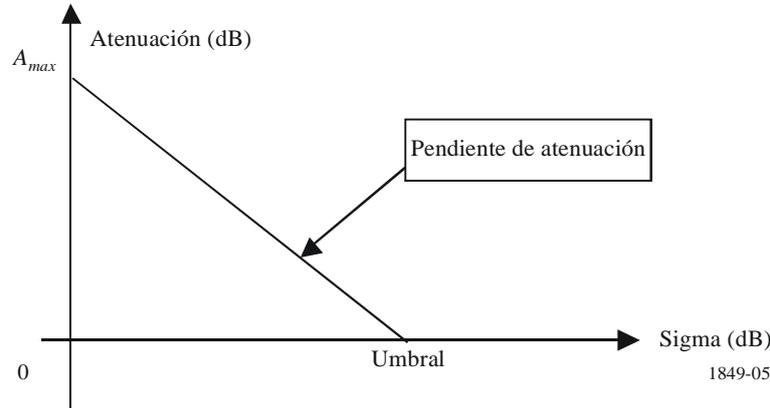
$$\text{Si } (\sigma \leq \text{Umbral}) \Rightarrow Z_{aeef} = Z_{seef} - (\text{Umbral} - \sigma) * \text{Pendiente}$$
